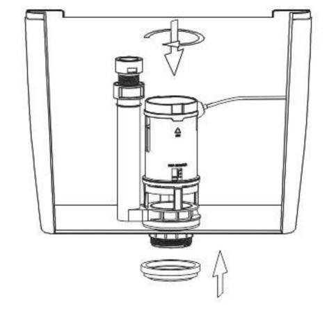
4. Take the body of flush valve and set it into the base and lock in place by rotating it clockwise. Then Insert the tank to bowl rubber gasket on to the flush valve's outlet bottom.
