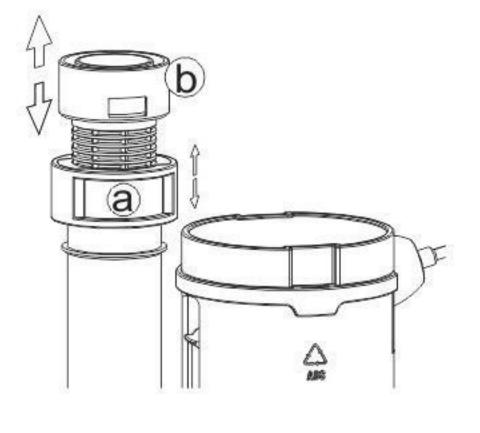
6. To adjust the height of the overflow pipe, slide the lock (a), then set the desired height of the overflow pipe (b). Put the lock back after.
