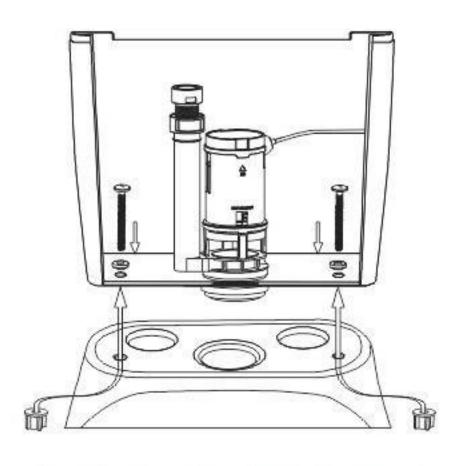
5. Fasten the tank to bowl with one pair of plastic or stainless steel bolts.Make sure bolts have the black rubber washer under the bolt's head.
