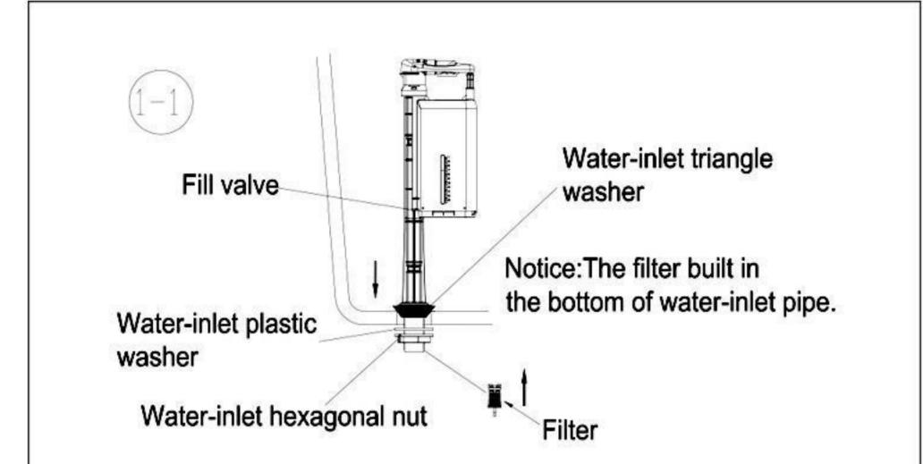
Put fill valve & water-inlet triangle washer insert into water-inlet hole of water tank, then, cover water-inlet plastic washer and hexagonal nut in turn from the bottom of fill valve. Fastening water-inlet hexagonal nut and make a proper adjust according to the size of water tank.
