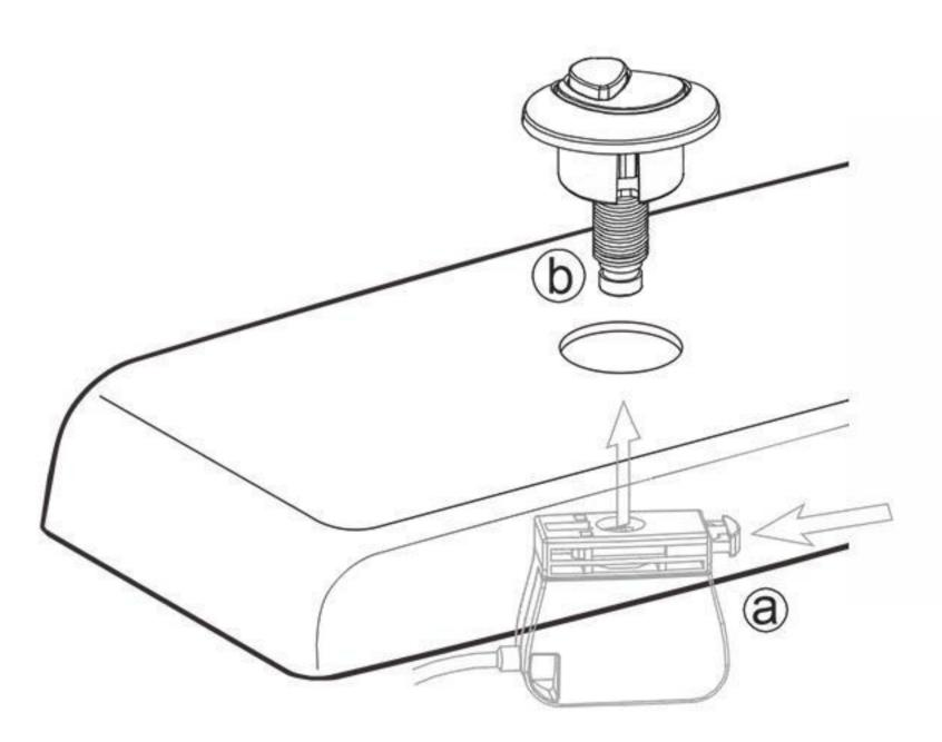
3. Push in the spring lock (a) which is on the control box and then insert button (b) into the control box.
